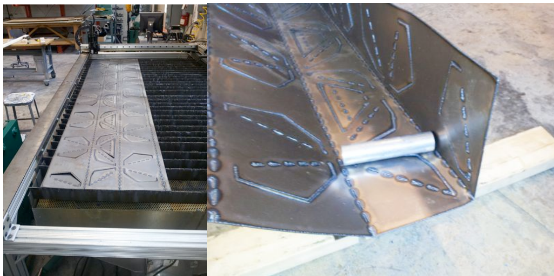
Figure 20. Construction process, cut sheet and jig for easy construction
