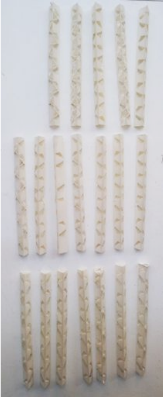
Figure 11. Small set of paper models which were tested under uniform loads.
