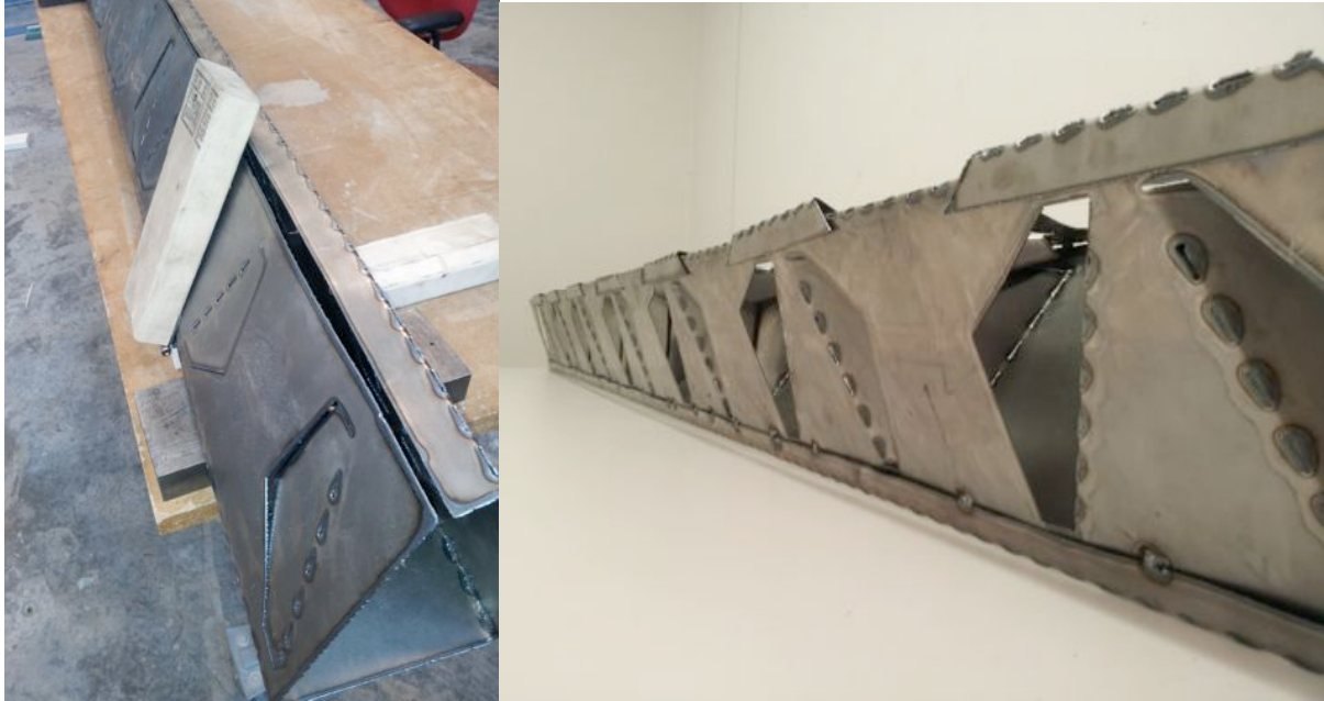
Figure 21. Profile folding process and final folded truss.
