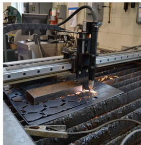
◀ Figure 8. CNC plasma cutting in progress.
